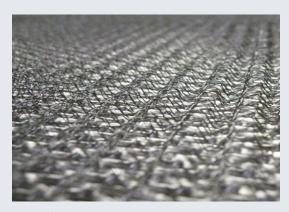
Knitex® Shielding Tapes can be produced with a crimp for greater thickness.
