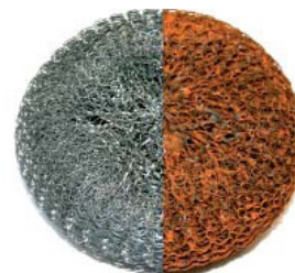
Leading competitor's scourer before and after corrosion testing
