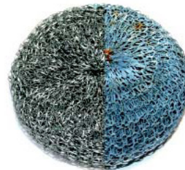
KleenKnit™ scourer before and after corrosion testing
