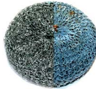
KleenKnit™ scourer before and after corrosion testing
