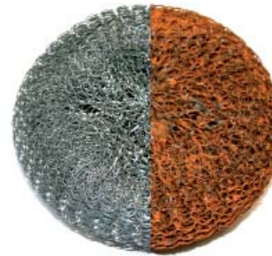
Leading competitor's scourer before and after corrosion testing
